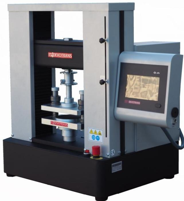
UTILISÉ POUR LES ESSAIS ECT, FCT, RCT, CMT, CCT ET PAT
