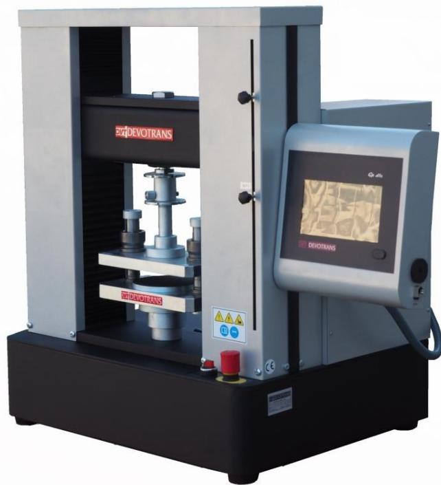
**USED FOR ECT, FCT, RCT, CMT, CCT, AND PAT TESTS**
